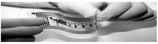
Figure 1: Medical RFID tag<sup>1</sup>
