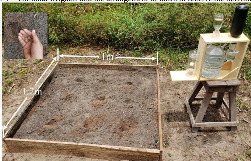
Figure 4 – The solar irrigator and the arrangement of holes to receive the beetroot seeds.
