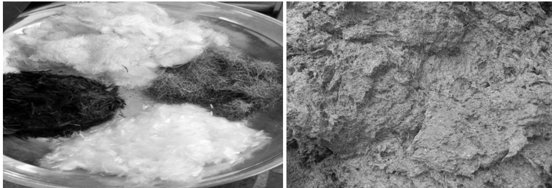
Figure 2: Fibers (Before and after mixing)
