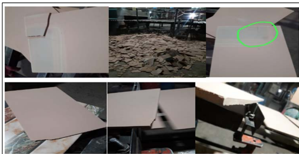
Figure 7: Defective and rejected tiles receive from bisque kiln
