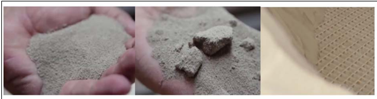
Figure 4: Slip powder formation in the spray dryer operation.
